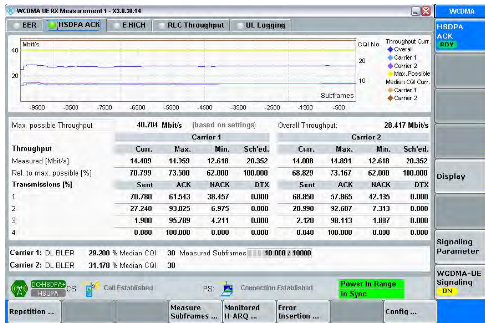
Fig. 4-29: WCDMA RX measurement for DC-HSPA. The measurements are adapted automatically for both streams individually and for the overall assessment.
