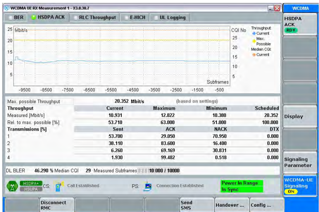
Fig. 4-10: WCDMA RX measurement for SISO.
